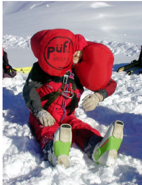
Fig.3 Measurement dummy with Avagear rescue vest
